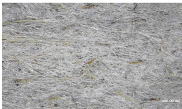
Figure 1 Aligned alkali treated fiber mat produced by dynamic sheet forming (DSF). [Color figure can be viewed in the online issue, which is available at wileyonlinelibrary.com .]
